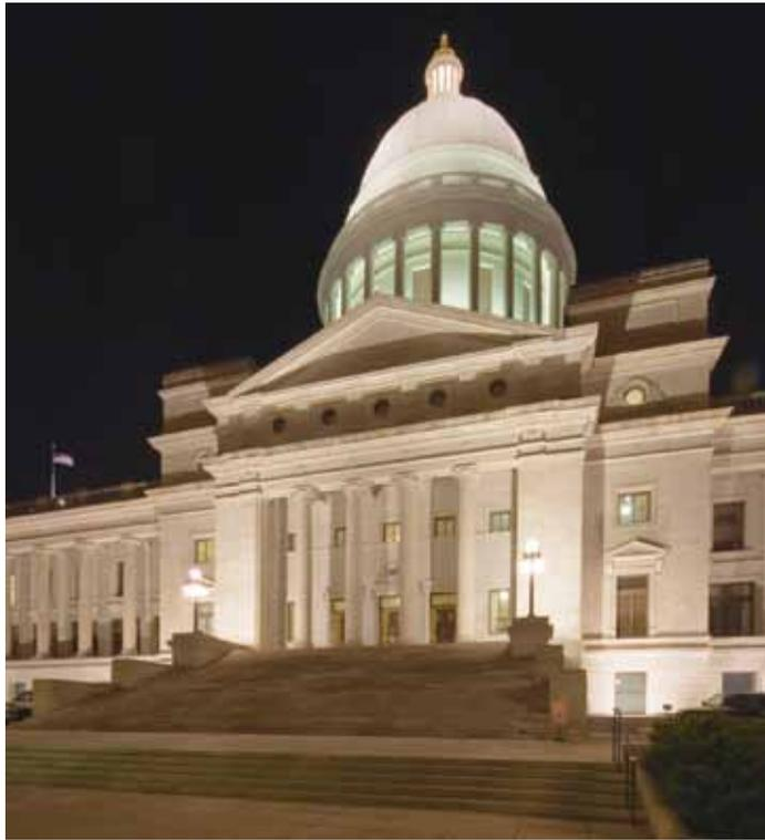
4000K CMH units were introduced at the main entry, where the grand stair interrupts the typical fixture spacing.
