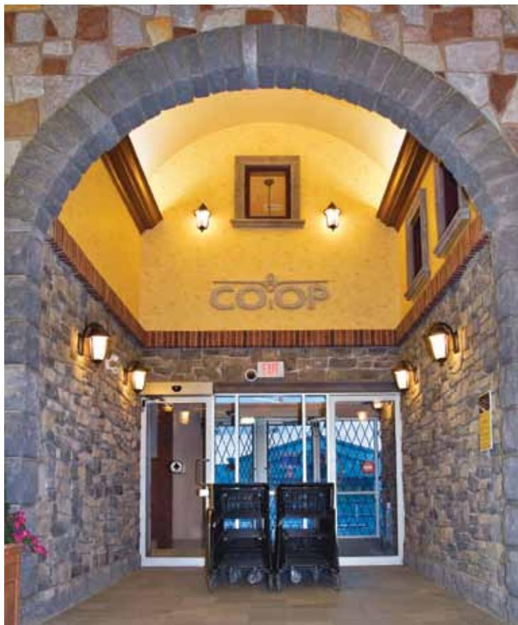
**elliptipar Style F305** fixtures with a single T5HO reflector light the vaulted ceiling at the entrance from coves above the clerestory. The even wash of light creates a welcoming glow to greet customers.
