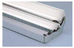
The integrally ballasted, dual T5HO **Style F308** offers versatile cove lighting for large spaces. The large upper reflector maximizes asymmetric performance and can be aimed lower for longer throws. Each row of reflectors can be aimed together and secured with locking set screws.
