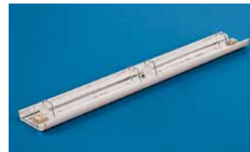
fraqtir's proprietary optic uses refraction and total internal reflection (TIR) to channel and transform light from a linear LED array into a smooth asymmetric distribution.
