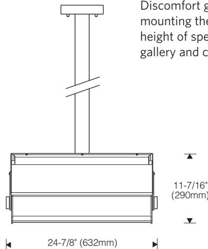
Discomfort glare is minimized by mounting the uplights above the eye height of spectators on the upper level gallery and corridor.
