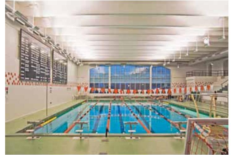
**After:** Working in concert with lighter finishes, indirect **M104** uplights illuminated the natatorium without direct or reflected glare.
