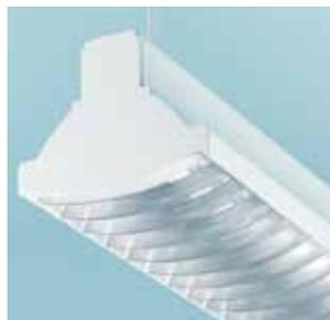
Semi-specular parabolic cross baffles in the **Style 3030** provide 25° shielding along the aisle. Optional occupancy sensors are positioned between baffle blades in designated fixtures.
